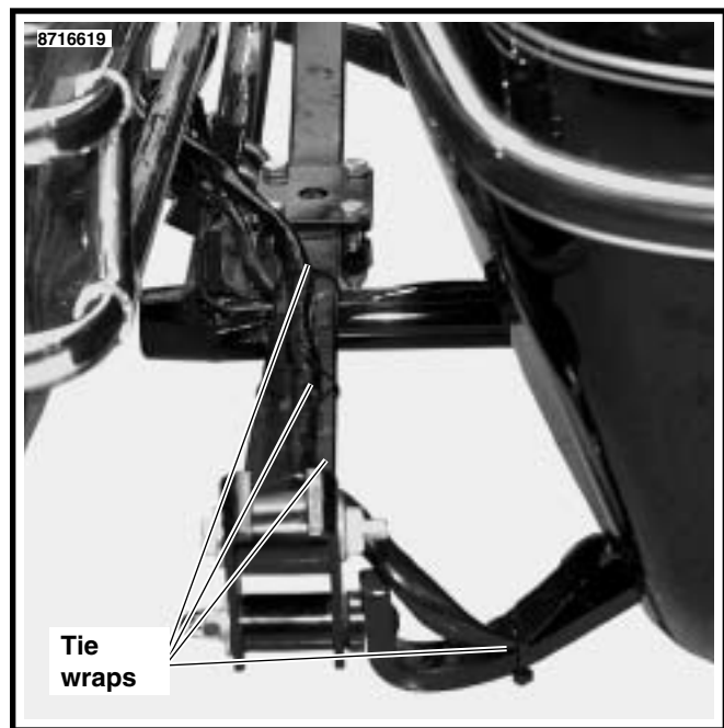
Figure 21. Sidecar Harness Routing
